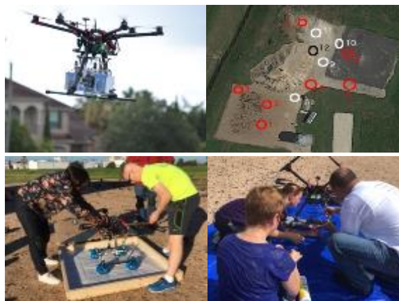
Figure 1: Upper Left: The Team Hexplorers hexacopter performing a sample collection sortie. Upper Right: Google Earth view of the JSC “Mars Yard” showing sites suitable for collecting representative samples from each “geological unit” present (red), simulated evaporite (white), and kerogen deposits (black). Lower Left: Team Ripsaw servicing their hexacopter between sampling sorties, showing the clean landing pad with single-use plastic liners for contamination control. Lower Right: Team RASCALS preparing for a sampling
