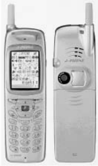
Figure 2.7 Sharp's SH-04 for J-Phone (2000), the first camera cell phone. Reproduced with permission.
